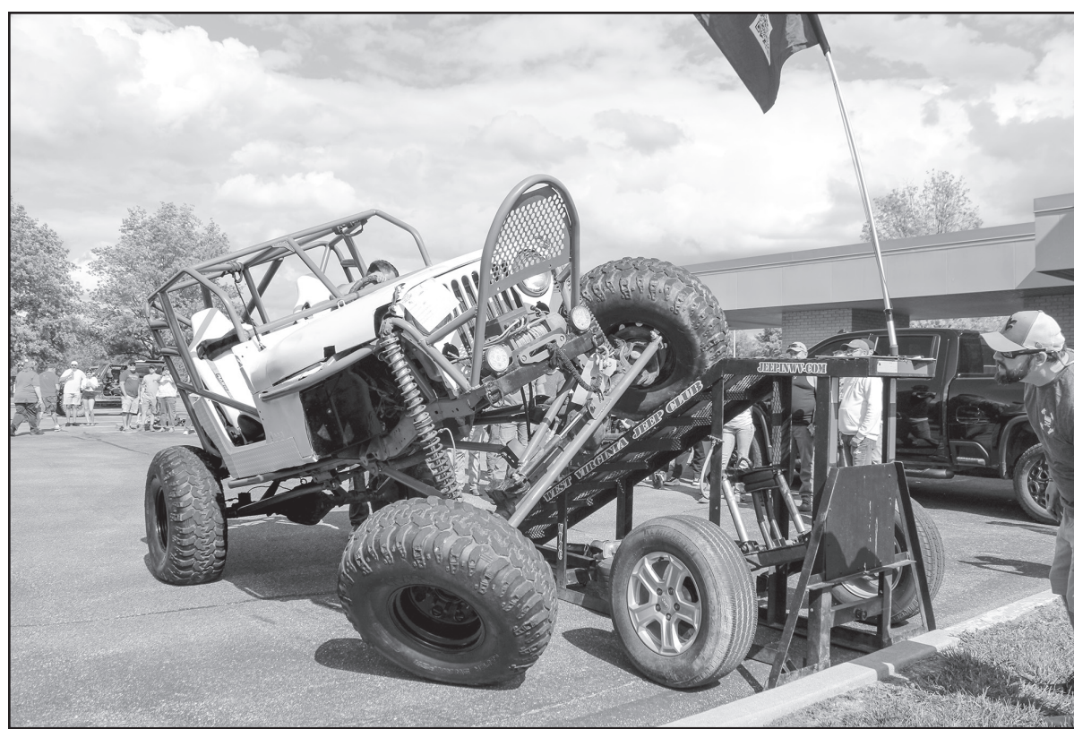
Justin Boyle of Hurricane takes his 1986 CJ-7 Jeep up the RTI ramp, which is used to determine a vehicle's suspension articulation.
