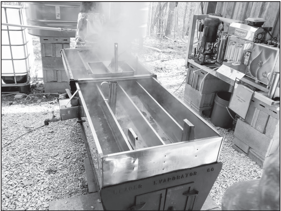
Paul Ronk's wood-fired evaporator can produce one gallon of syrup per hour.
