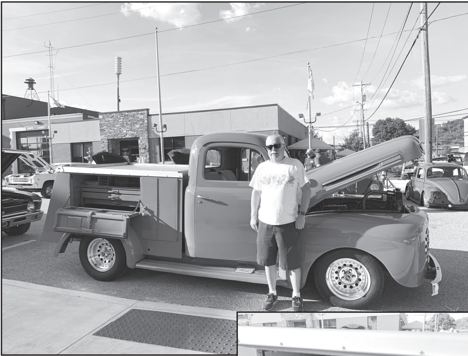
Andrew Wallace of Milton shows off his bright blue 1948 Ford telephone utility truck. The truck features various cubbies and a set of drawers with sectioned off dividers which were used to store telephone terminals and other equipment. These features are accessed on the passenger's side, so that the driver would not have to walk out into traffic to get supplies. At one time, the truck was equipped with ladders on both sides. In the 1960's, phone companies switched over to using vans instead of these special utility trucks. (Photo by Betsy Allen)
